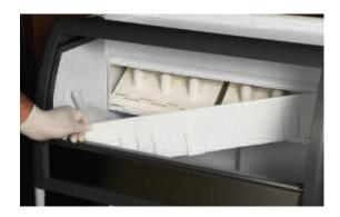
5. Lift up and remove the curtain. (No curtain is fitted on the AC/EC 206 & 226)
