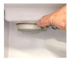
5. Lift up curtain from brackets and remove the same.
