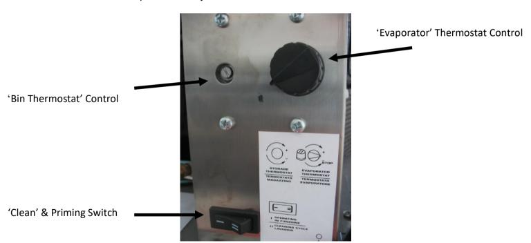
• NOTE – During install/commissioning, adjust the 'Bin Stat' control fully clockwise to prevent nuisance tripping off under a bin full condition...
