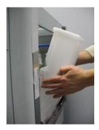
On the MC Range remove the plastic sump cap of the sump to drain the unit
