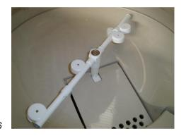
Lift up and remove the spray bar from its seat/spigot and take out to clean it separately along with the perforated tray of the sump chamber.
