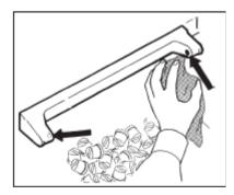
Wipe clean and rinse the inner surfaces of the storage bin using an appropriate sanitising product along with the cleaning of the ice level sensor lenses on the inside of the unit storage bin.
