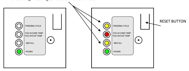
**NOTE.** With the system in CLEANING/RINSING mode, the water pump is the only component in operation to circulate the cleaning solution in the entire water system while the three LED's of the PC Board are blinking.
