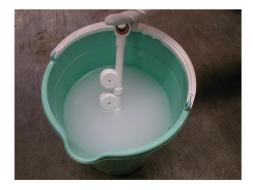
Install again the spray bar & washer, as well as the bottom perforated tray before moving to a full system descale or sanitise.
