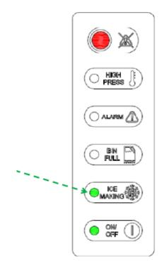
When the water tank is full, the machine should now start an ice making cycle (this after approx 2 minutes) with the compressor in operation.
