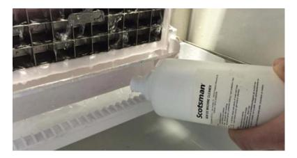
.....the water inlet valve will be energized till the fill up of the water sump. The water pump starts to operate
