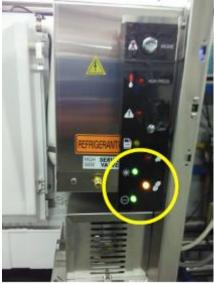
Following a short period of harvest, approx. 2 minutes, a sheet of ice should fall through the curtain and into the storage bin. The machine should then automatically refill with water and start the next cycle.
