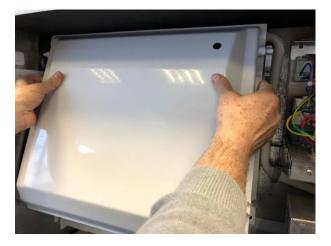
Unscrew water pump bracket screws and remove it from the reservoir
