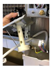
Unscrew the two thumb screws then withdraw reservoir from its seat
